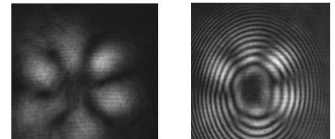
Fig. 8: A sinusoidal LG<sub>0</sub><sup>3</sup> mode shows a striated petal pattern and an offset in the first three interference rings.
