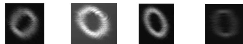
Fig. 5: Arbitrary high order LG modes: LG<sub>5</sub><sup>0</sup>, LG<sub>6</sub><sup>0</sup>, LG<sub>7</sub><sup>0</sup>, LG<sub>8</sub><sup>0</sup>
