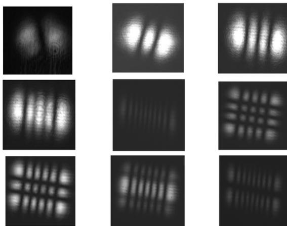
Fig. 1: HG<sub>0</sub><sup>1</sup>, HG<sub>0</sub><sup>2</sup>, HG<sub>0</sub><sup>3</sup>, HG<sub>0</sub><sup>4</sup>, HG<sub>0</sub><sup>9</sup>, HG<sub>4</sub><sup>3</sup>, HG<sub>5</sub><sup>2</sup>, HG<sub>6</sub><sup>2</sup>, HG<sub>8</sub><sup>1</sup> modes
