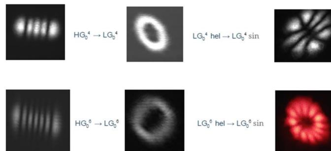
Fig. 6: Full HG to LG<sub>hel</sub> to LG<sub>sin</sub> conversion
