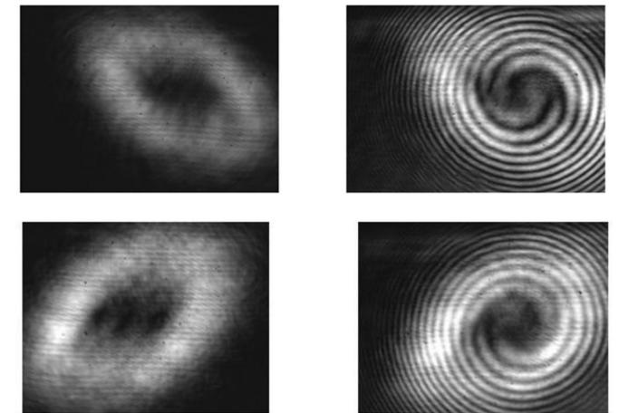
Fig. 7: Oppositely handed helical LG modes with their resultant phase patterns. Counter clockwise and clockwise spirals respectively. The number of spirals corresponds to the order of the mode.
