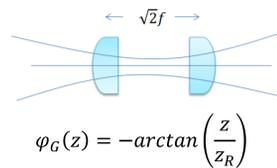
The first cylindrical lens introduces an astigmatism and definite phase difference (π/2) between HG components oriented along axes of astigmatism. The second cylindrical lens removes the astigmatism, leaving a modal beam which has a constant intensity distribution throughout propagation.
