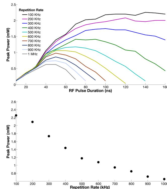
Peak power per pulse is related to RF signal duration and repetition rate. Output pulse duration stays constant at about 100 ns.
