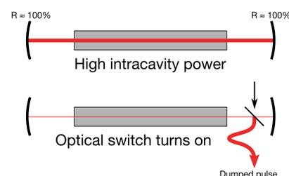
With cavity dumping, the OC is replaced with an HR to enable high intracavity power. Intracavity power is repetitively deflected out of the cavity by a high speed optical switch like an acousto-optic modulator or electro-optic modulator.
