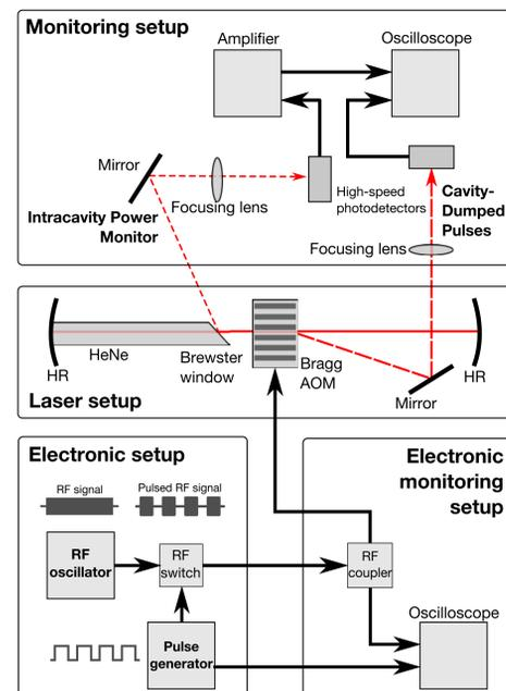
The cavity is 1.4 m in length. Clipping the cavity-dumped beam out of shorter cavities was not possible without blocking the intracavity beam.
