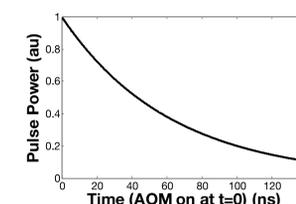
This model predicts a pulse duration (fwhm) of ~50 ns. Pulse broadening and the symmetrical shape were caused by the rise/falltime of the RF pulse, and the acoustic beam transit time across the laser beam.
