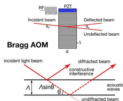
A Bragg AOM diffracts an incident beam into a single first order beam.
