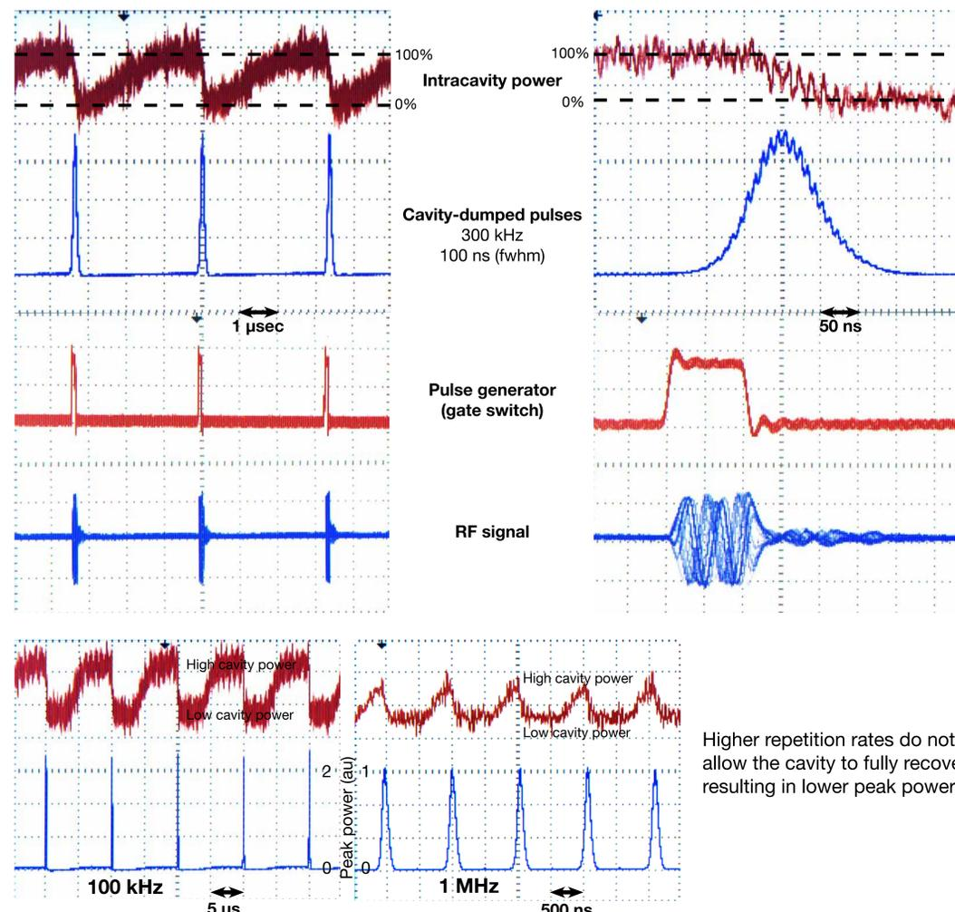
Higher repetition rates do not allow the cavity to fully recover, resulting in lower peak powers.
