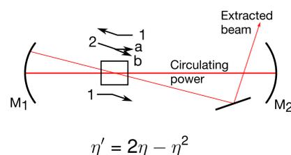
For an AOM placed at the cavity beam waist, double-pass diffraction efficiency ( $\eta'$ ) depends on single-pass diffraction efficiency ( $\eta$ ). We were, however, not able to recapture the return beam.
