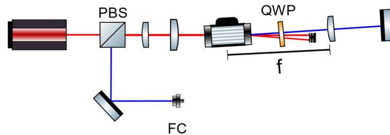
PBS= Polarizing beam splitter FC= Fiber coupler QWP= quarter-wave plate to select the frequency shifted light on its return path through the PBS.
