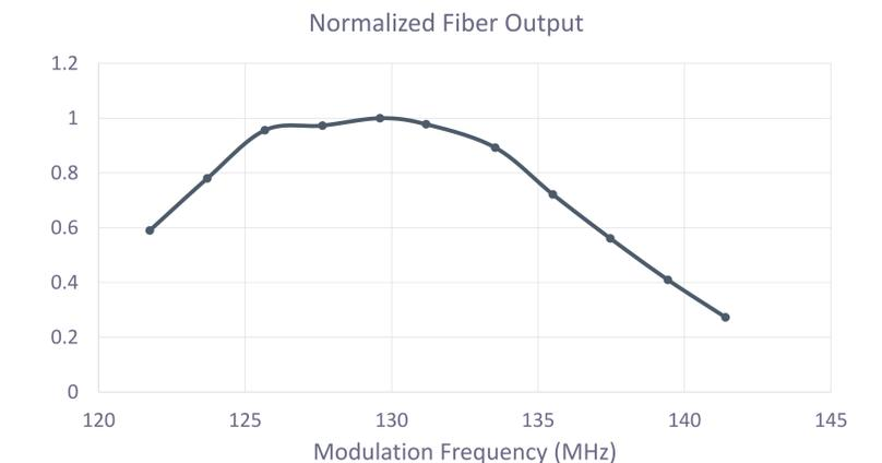
Coupling efficiency is quite good over our frequency range of interest (FWHM>20MHz). The asymmetry in the curve implies that there was a misalignment but due to time constraints, a better alignment was not recorded.
