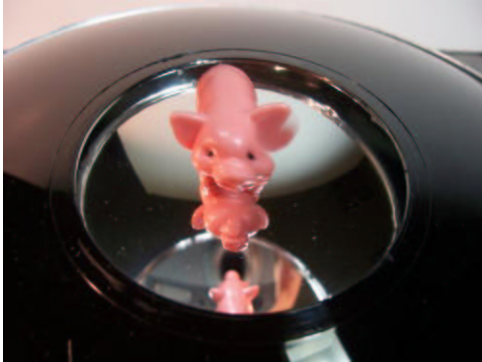
Figure 1: Photograph of the Opti-Gone Mirage ® in our laboratory showing, from top to bottom, the projected real image, the projected reflection, and the actual object. The two images appear larger than the actual object primarily because the camera is close to the device. [Photo courtesy Azure Hansen.]
